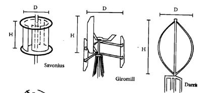
Diagram of different rotors for horizontal and vertical axis wind turbines.
