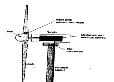
Main parts of a utility-scale wind turbine
